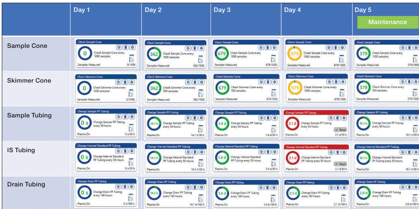
Figure 1. Detailed maintenance requirements for different parts in the ICP-MS system
