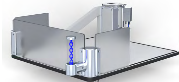
Figure 4: The Thermo Scientific™ Spinnaker™ XT robot is the central mover to the inSPIRE platform, and it is responsible for microplate transportation between all instruments on the system.
