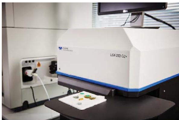
FIGURE 1. Combined LSX-213 G2+ / iCAP Q LA-ICP-MS system
