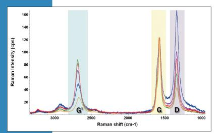
Figure 2: Raman spectra of 95% pure multiwall carbon nanotubes of different diameters ranging from < 8 nm to > 50 nm measured with 0.5 mW of excitation laser power
