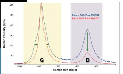
Figure 1: Comparison of the Raman spectra of 60% and 90% pure single-wall carbon nanotubes
