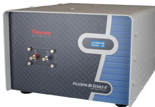
picoSpin 80 Series II NMR spectrometer
